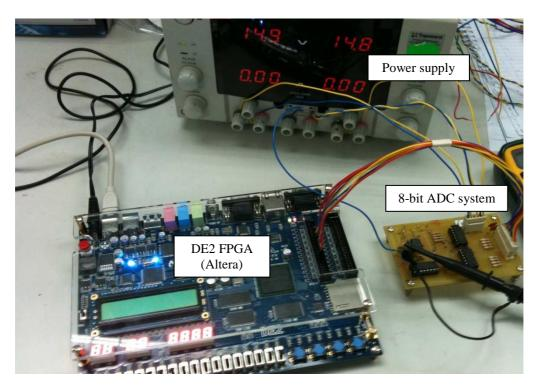
Figure 4. Experiment setup
